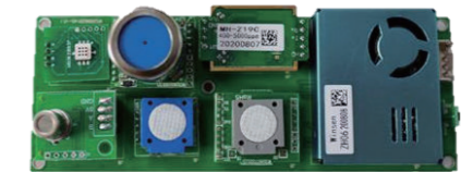
ZPHS01B 9-in-1 Air Quality Detection Module (CO 2 , PM2.5/10, TVOC, CO, O 3 , CH 2 O, NO 2 , T&H)
