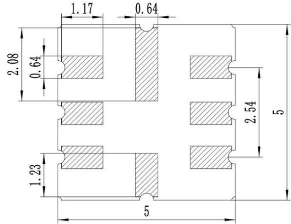
Bottom Apparent size (Unit: mm)
