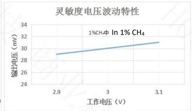
**Fig10.Sensitivity with different voltage**
