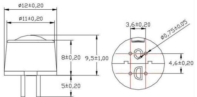
Fig1. Sensor Structure
