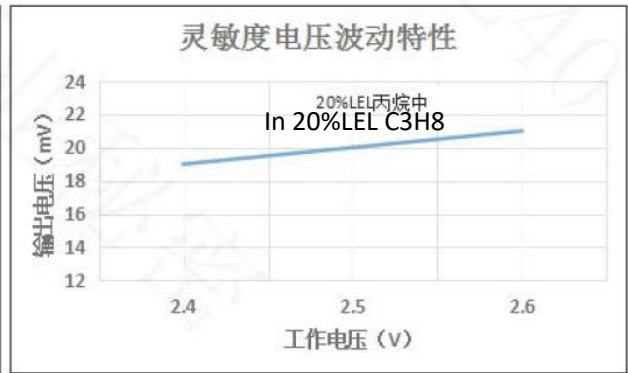
Fig10.Sensitivity with different voltage
