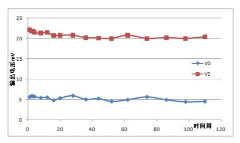
The absolute value of the drift in air is less than 2 mV per year, in 10%CH4 the absolute value of drift is less than 2mV. For a short period storage (in 2 weeks), the sensor need 8 hours preheating to stabilize, for long-term (more than one year) storage, it need more than 48 hours' preheating.
