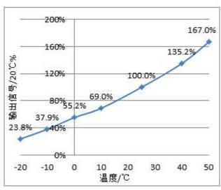
Sensor Zero Drift upon variable temperature
