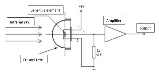
By using different Fresnel lens, the detection range and distance can be determined. According to customer's requirement, it can response to various detection range and distance.
