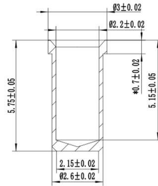
Fig2. Tube base dimension for module matching
