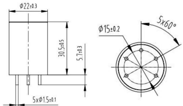
Fig1. Module side and bottom views
