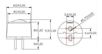
Fig1. Sensor Structure
