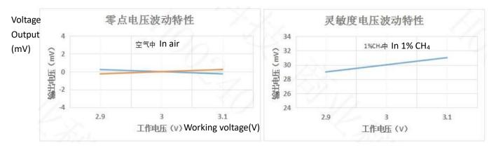
Fig9.Zero Drift with different voltage
