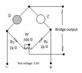
Fig2. Basic Test Circuit
