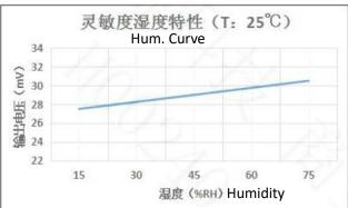
Fig7.Zero point at different humidity
