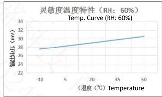
Fig5.Zero point at different temp.
