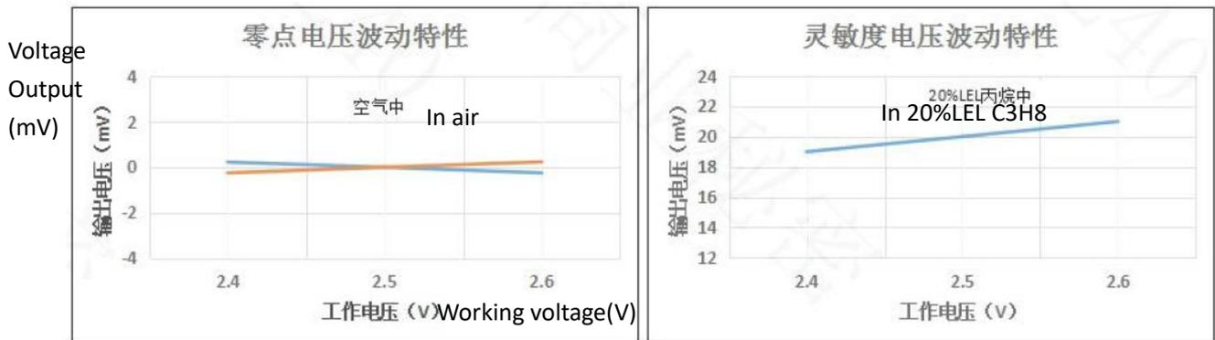
**Fig9.Zero Drift with different voltage**
