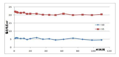
The absolute value of the drift in air is less than 2 mV per year, in 30%CO2 the absolute value of drift is less than 2mV. For a short period storage (in 2 weeks), the sensor need 8 hours preheating to stabilize, for long-term (more than one year) storage, it need more than 48 hours' preheating.
