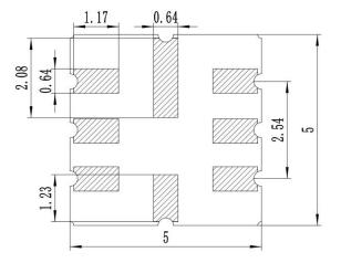
Bottom Apparent size (Unit: mm)
