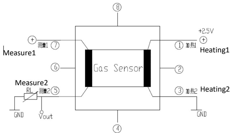
Instructions: The above fig is the basic test circuit of GM-502B. The sensor requires two voltage inputs: heater voltage ( $V_H$ ) and circuit voltage ( $V_C$ ).  $V_H$  is used to supply specific working temperature to the sensor and it can adopt DC or AC power.  $V_{out}$  is the voltage of load resistance  $R_L$  which is in series with sensor.  $V_C$  supplies the detect voltage to load resistance  $R_L$  and it should adopt DC power.
