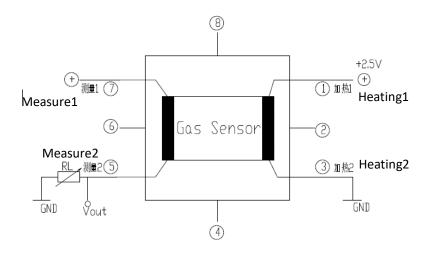
Instructions: The above fig is the basic test circuit of GM-502B. The sensor requires two voltage inputs: heater voltage ( $V_H$ ) and circuit voltage ( $V_C$ ).  $V_H$  is used to supply specific working temperature to the sensor and it can adopt DC or AC power.  $V_{out}$  is the voltage of load resistance  $R_L$  which is in series with sensor. Vc supplies the detect voltage to load resistance  $R_L$  and it should adopt DC power.
