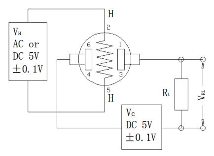
Fig2. MQ136 Test Circuit
