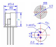
Fig1.Sensor Structure (Unit: mm)
