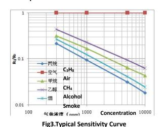
The ordinate is resistance ratio of the sensor (Rs/R<sub>0</sub>), the abscissa is concentration of gases. Rs means resistance in target gas with different concentration, R<sub>0</sub> means resistance of sensor in clean air. All tests are finished under standard test conditions.
