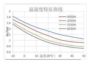
Fig4.Typical temperature/humidity characteristics
