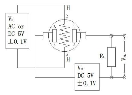
Fig2. MQ-2 Test Circuit
