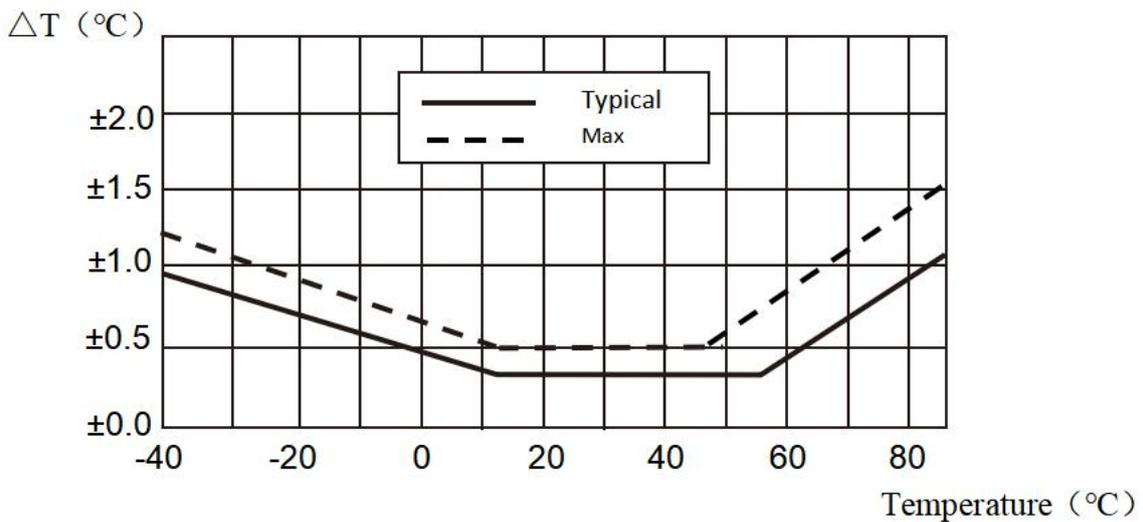
Figure 2 Temperature typical error and maximum error
