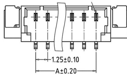
**Fig2.**Part no. of Pins(A=8x1.25)
